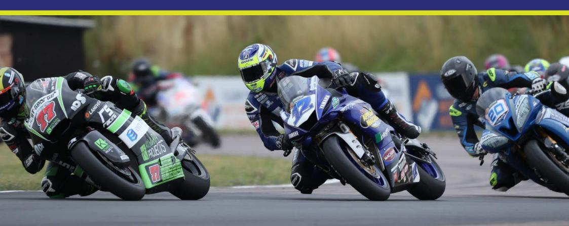
After a lengthy post quali de brief we again made some fairly big changes for the race. We dropped one tooth on the rear sprocket to allow me to use 4th gear on the fast parts of sector 2 which would give me the drive I was after. In contrast, by dropping a tooth you lengthen the wheelbase.
